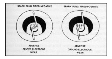
Due to the ever-increasing cost of aircraft maintenance and a desire to get the maximum service life from your spark plugs, the following information is offered on the effects of constant polarity and how to rotate plugs to get maximum service life.
